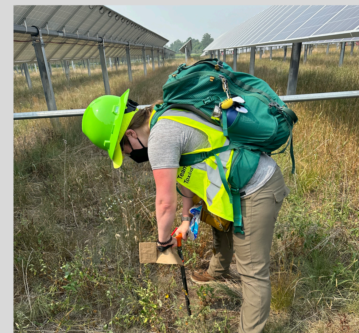
Figure 2: demonstrates collecting soil samples.
